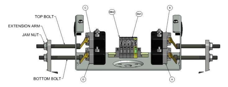
NOTE: BRAKES MUST BE INSPECTED DURING NORMAL ELEVATOR MAINTENANCE. IF LININGS INDICATE WEAR, THEN SPRINGS, GAPS AND MONITOR SWITCH MUST BE READJUSTED ACCORDINGLY.
